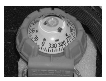
We must be careful where we position our compass on our flight deck. Any nearby magnetic material will cause it to misread. Other instruments and radios are likely to have magnetic material in them. Some batteries can be magnetic.
